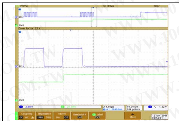
FIGURE 2-18: 5 k \Omega – Low-Voltage Increment Wiper Settling Time ( V_{DD} = 2.7\text{V} ) (1 \mu\text{s}/\text{Div} ).
