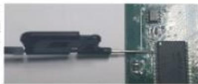
2: After use, don't force the clip off from the chip pin. To push out the clip and gently remove it from the chip pin.
