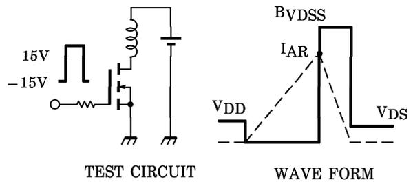
Peak  $I_{AR} = 3A$ ,  $R_G = 25\Omega$      $E_{AS} = \frac{1}{2} \cdot L \cdot I^2 \cdot \left( \frac{B_{VDSS}}{B_{VDSS} - V_{DD}} \right)$
