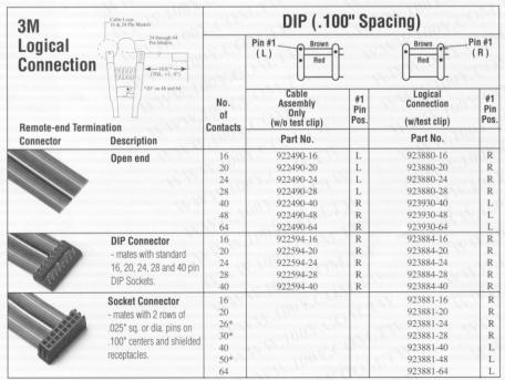
$<sup>\</sup>ast$  On 26 position connectors, positions #25 and #26 are unused. On 30 position connectors, positions #29 and #30 are unused. On 50 position connectors, positions #49 and #50 are unused.
