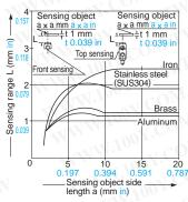
As the sensing object size becomes smaller than the standard size (iron sheet 15 x 15  $\times$  t 1 mm 0.591  $\times$  0.591  $\times$  t 0.039 in), the sensing range shortens as shown in the left figures.
