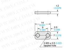
Material: Cold rolled carbon steel (SPCC)
