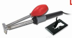
With a vacuum bulb and 45W of power, this desoldering iron makes it easy to remove molten solder while still keeping one hand free. Vacuum bulb pulls up molten solder.
