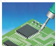
Soldering from 2 opposite angles
