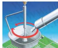
Desoldering IC component with hot air
