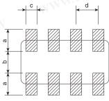
dimension for Reflow-soldering (unit: mm)
