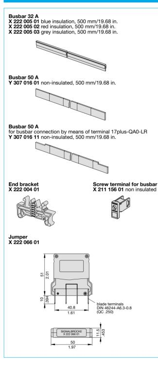
This is a metric design and millimeter dimensions take precedence (  $\frac{mm}{inch}$  )
