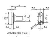
Actuator Mounting Hole Layout
