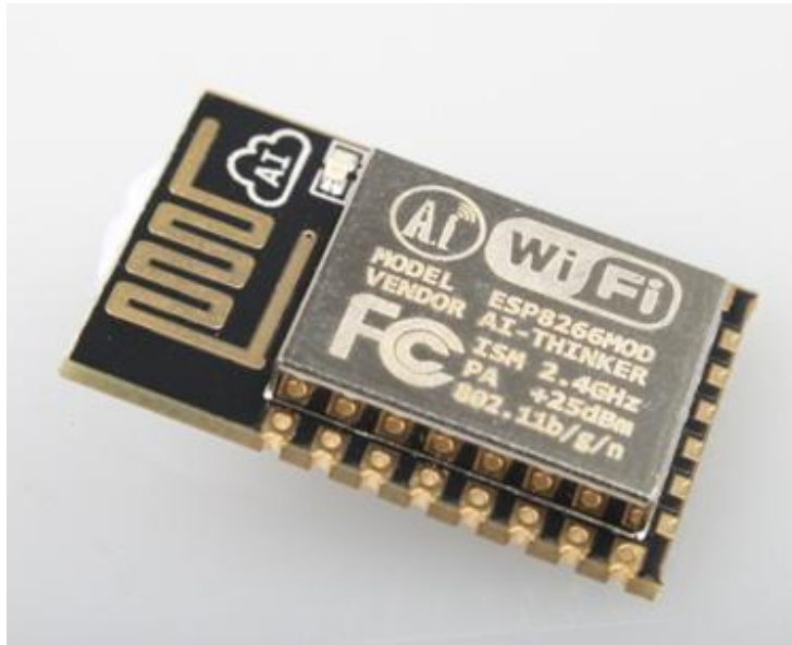
Figure 3 [Module Pin Counts, 22 pin, 16 mm *24 mm *3 mm]
