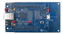
2. Plug the FMC Interconnect Board into the Xilinx® FPGA board (The Xilinx FPGA board is not part of this kit)
