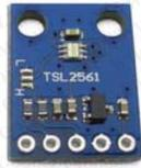
Description: The TSL2561 Luminosity Sensor Breakout is a sophisticated light sensor which has a flat response across most of the visible spectrum. Unlike simpler sensors, the TSL2561 measures both infrared and visible light to better approximate the response of the human eye. And because the TSL2561 is an integrating sensor (it soaks up light for a predetermined amount of time), it is capable of measuring both small and large amounts of light by changing the integration time
