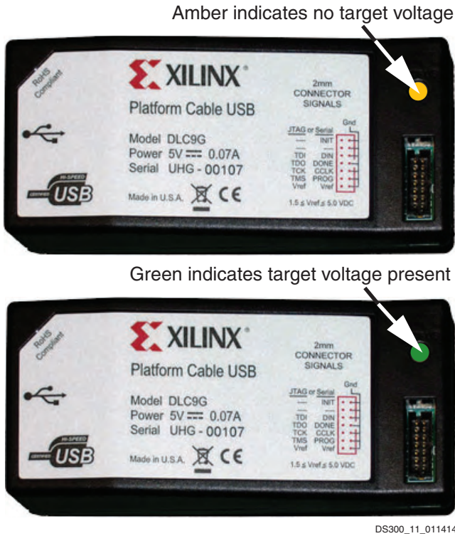
Figure 11: Status LEDs Indicating Target Voltage
