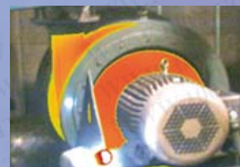
IR/Color Alarm Displays only temperatures falling above, below, or in between a user- selected range in infrared, and anything outside the selected range as a visual (visible light) image. (In software only.)
