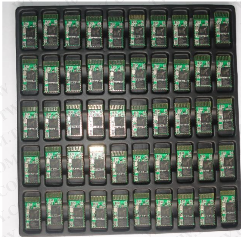
Figure 3 50 pieces chips in an anti-static blister package.
