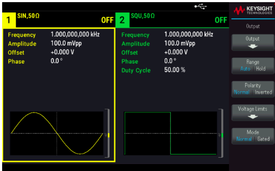
Figure 2. Dual-screen display of standard sine and square wave
