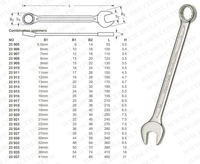
The specified B1, B2, L and H dimensions are within the tolerance required to meet DIN 3113.
