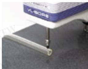
Diameter of resin pipe
