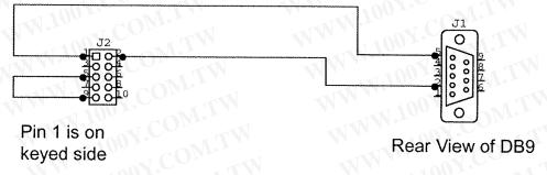
J2-1 Level Ground ==> J1-5 Computer Ground ==> J1-2 RX of Computer J2-2 TX of Level J2-5 RX of Level ==> J2-9 Batt+ of Level
