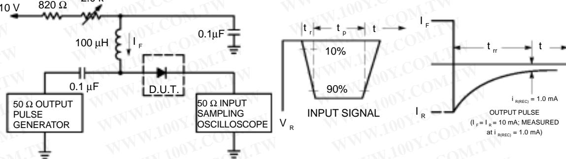
Notes: 1. A 2.0 kΩ variable resistor adjusted for a Forward Current ( $I_F$ ) of 10mA.
