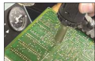
Through hole rework with the DSV80
