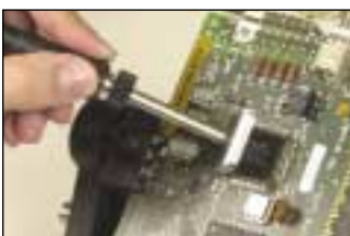
A SMT quad tip is used to desolder a quad flat pack with the WSP80 soldering pencil.
