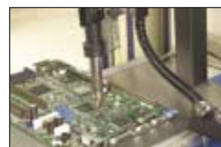
Step 3: The component is lifted off the board using the built-in vacuum pick-up.
