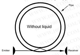
If there is liquid in the pipe, the emitted beam will pass through the liquid and not reach the receiver.
