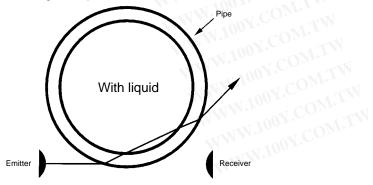
If the diameter of the pipe is close to 6 mm, some of the emitted light may reach the receiver because the angle of refraction is small. This may result in false readings. In such cases, set the sensitivity selector to Low and check that the EE-SPX613 reads correctly for pipes with and without liquid.
