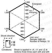
Shock is applied in  $\pm X, \pm Y$ , and  $\pm Z$  directions three times each with and with out energizing the Relays to check the number of contact malfunctions.
