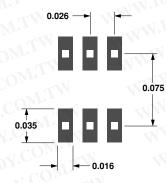
Figure 7. PCB Pad Layout (dimensions in inches).
