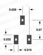
Figure 6. PCB Pad Layout (dimensions in inches).
