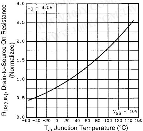
**Fig 4.** Normalized On-Resistance
