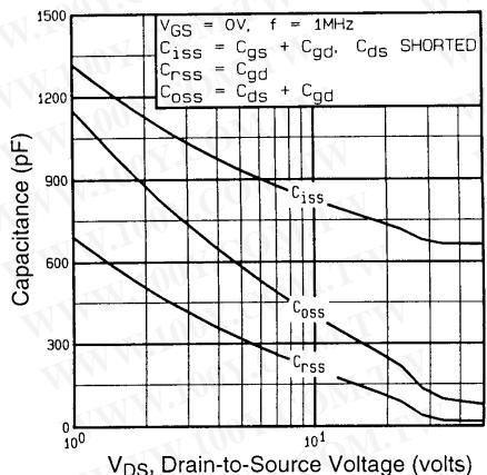
Fig 5. Typical Capacitance Vs.
