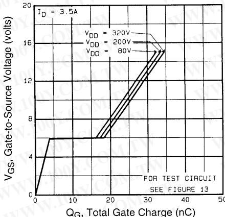
Fig 6. Typical Gate Charge Vs.
