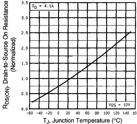
Fig 4. Normalized On-Resistance
