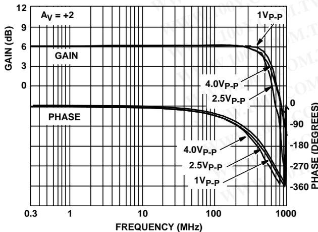
FIGURE 13. FREQUENCY RESPONSE FOR VARIOUS OUTPUT VOLTAGES
