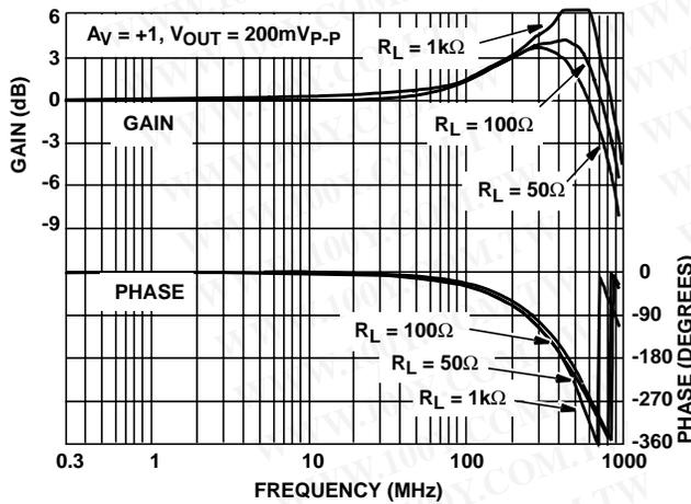
FIGURE 11. FREQUENCY RESPONSE FOR VARIOUS LOAD RESISTORS
