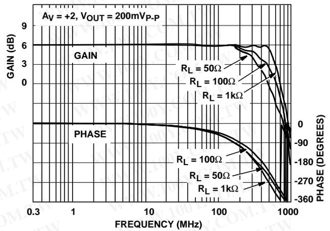
FIGURE 10. FREQUENCY RESPONSE FOR VARIOUS LOAD RESISTORS
