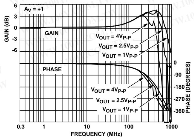
FIGURE 14. FREQUENCY RESPONSE FOR VARIOUS OUTPUT VOLTAGES
