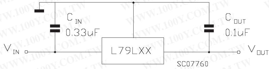
**CONNECTION DIAGRAM AND ORDERING NUMBERS (top view)**
