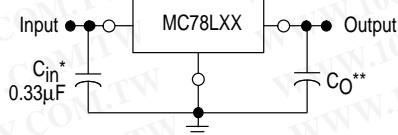
A common ground is required between the input and the output voltages. The input voltage must remain typically 2.0 V above the output voltage even during the low point on the input ripple voltage.
