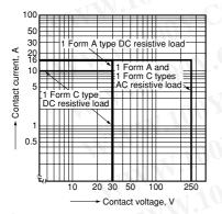
1-(2). Max. switching capacity (2 Form C)
