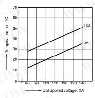
2-(3). Coil temperature rise (2 Form C/AC type) Measured portion: Inside the coil Ambient temperature: 70°C 158°F
