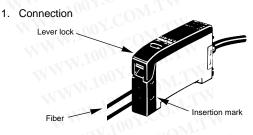
Insert the fibers into the E3X amplifier and press the lever lock until the amplifier clicks to lock the fibers. The fibers will have insertion marks when they are cut with the E39-F4 (Fiber Cutter). The portion from the tips to the insertion mark should be inserted to the E3X.
