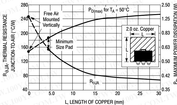
Figure 10. SOT-223 Thermal Resistance and Maximum Power Dissipation versus P.C.B. Copper Length
