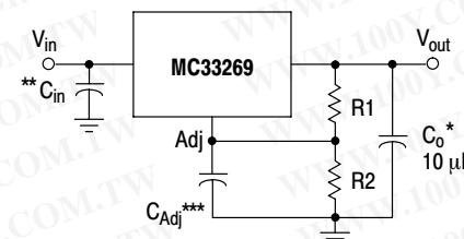
$$V_{\text{out}} = 1.25 \left( 1 + \frac{R_2}{R_1} \right) + I_{\text{Adj}} R_2$$
