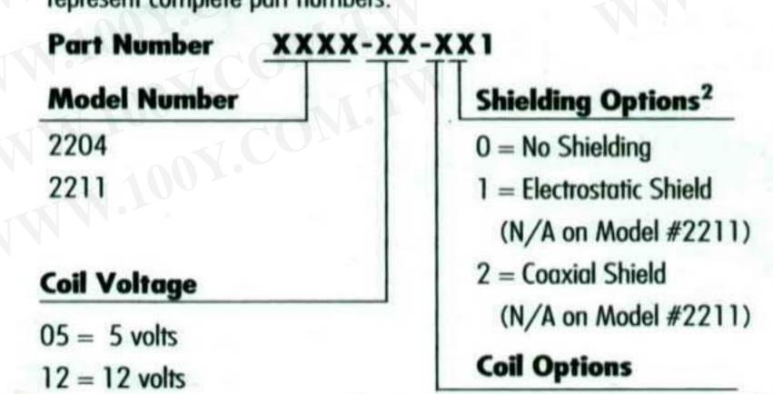
3 = use for Model # 2204 (12 volt coil) and Model # 2211 (5 & 12 volt coil) 4 = use for Model # 2204 (5 volt coil)
