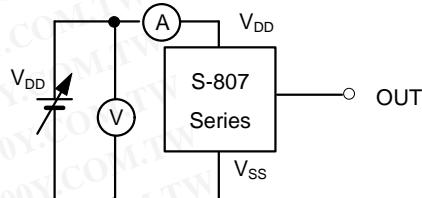
(3) Output transistor current
