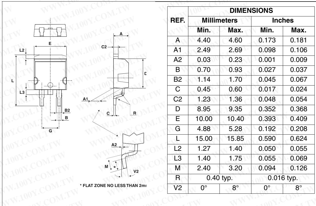
**Figure 14: Foot Print Dimensions (in millimeters)**
