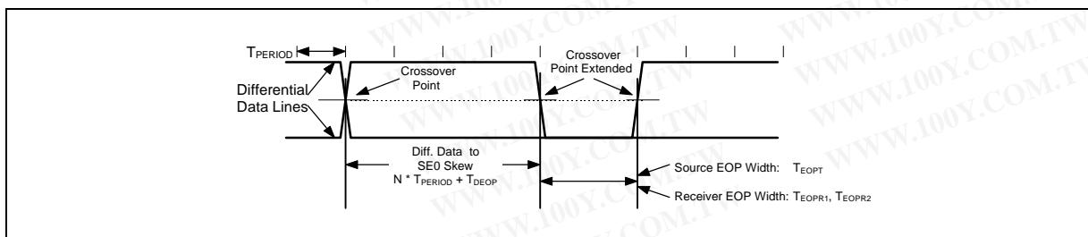
Figure 9.3 Differential to EOP Transition Skew and EOP Width
