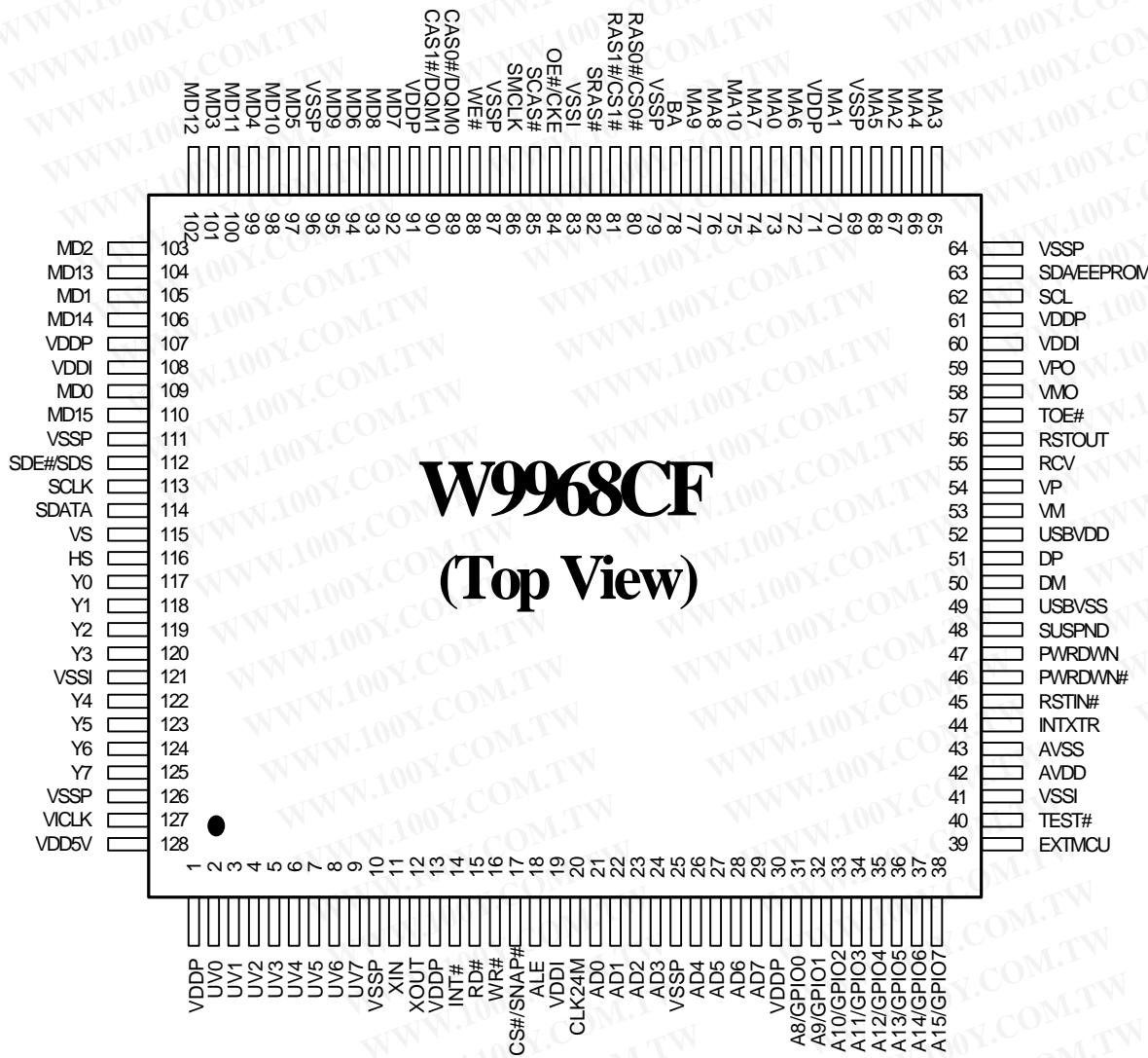
Figure 3.1 W9968CF Pin Configuration
