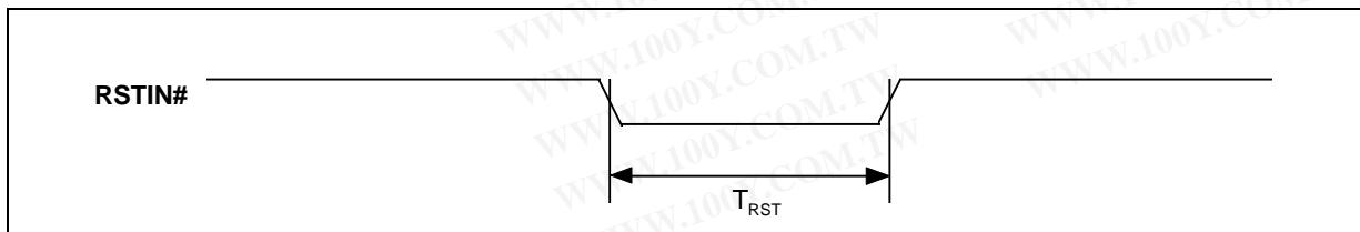
Figure 9.5 RESET Timing
