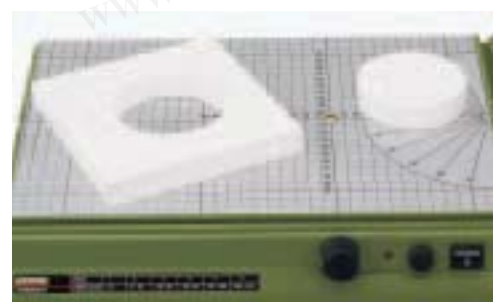
Crosscuts are achieved by means of a simple yet efficient solution: Secure drawing-pin to table by means of tape, it serves as a fixed centre.
